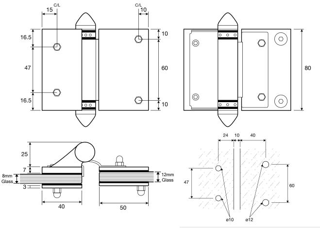
glass hole req. for top and bottom of glass panel and gate
