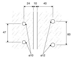
glass hole req. for top and bottom of glass panel and gate
