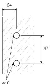
glass hole req. for top and bottom of glass gate
